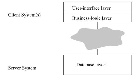
c) A three-layer approach that can also be used as an alternative to the thin client approach. (Note that the client would never see any difference between this approach and the thin-client approach; in fact, many e-commerce systems are in fact built this way)
