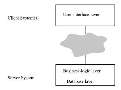
b) The so-called "thick client" approach, used when it is desirable to install the business logic software on the client system (This wouldn't work for e-commerce, of course, but is sometimes used for specialized applications)
