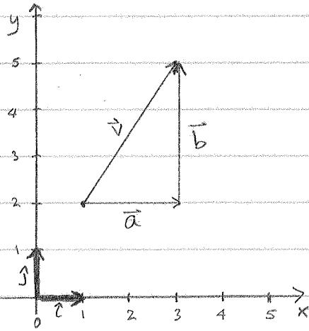
If we agree to define the addition of two vectors by placing one vector's tail on the other's head and let the sum be the vector from the tail of the first vector to the head of the second then  $\vec{v} = \vec{a} + \vec{b}$ .
