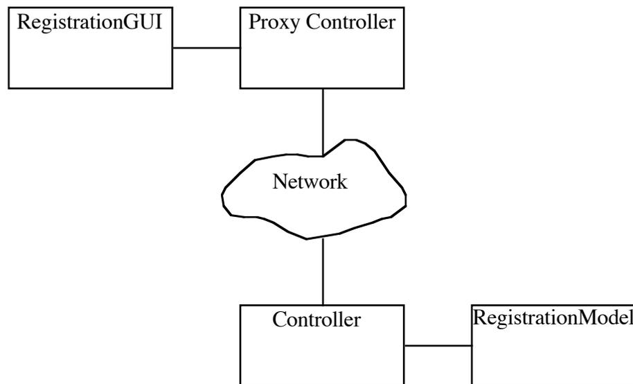
1. The proxy controller running on the remote computers has the same interface (the same set of methods) as the “real” controller running on the main computer.
